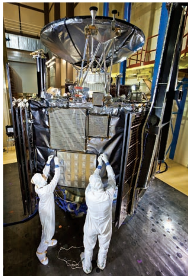
Technicians at a Lockheed Martin Space Systems facility in Denver, Colorado, inspect the Juno spacecraft after a simulation of the acoustic and vibration environment it will experience during launch. Credit: Lockheed Martin
