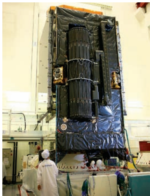
Alphasat I-XL uses a new deployable dish antenna technology. The Alphasat I-XL dish will be 12 meters (39.4 feet) in diameter and will augment Inmarsat's mobile data and voice services, increasing capacity across Europe, Asia, Africa, and the Middle East. Credit: Astrium
