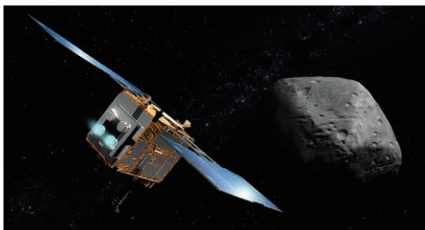
A possible new function of Hayabusa 2 would be to send an impactor to create a crater on an asteroid. This would enable the collection of samples that have not been exposed to the space environment to the same degree as the asteroid's surface. Credit: Akihiro Ikeshita
