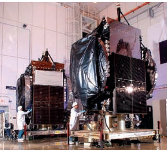
In addition to its commercial payload, the SES-2 communications satellite also includes the Commercially Hosted Infrared Payload (CHIRP) for the U.S. Air Force. Benefits of hosted payloads include increased cost effectiveness and more flexible flight opportunities. Credit: Orbital Sciences
