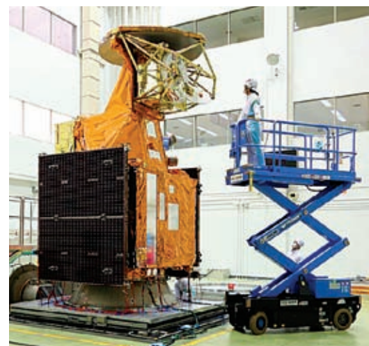
A JAXA technician inspects the Global Change Observation Mission Water (GCOM-W1) satellite after a vibration test. NOAA has negotiated a data-sharing partnership with JAXA to use information from the satellite for weather forecasting. Credit: JAXA
