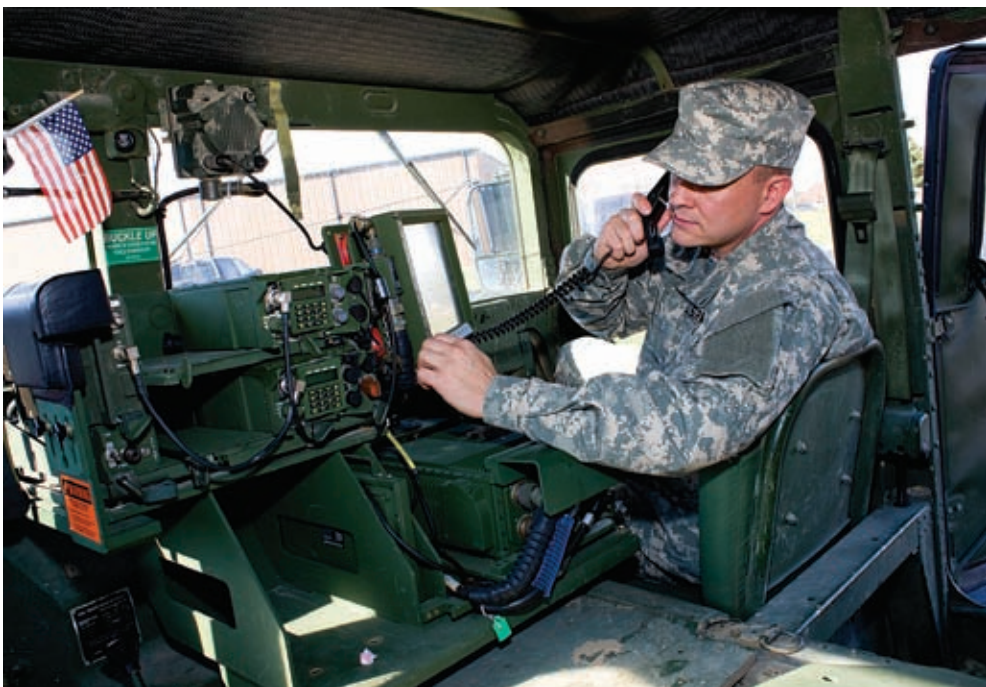
A GPS receiver embedded in the SINCGARS tactical radio, manufactured by ITT Exelis, provides U.S. troops with positioning, navigation, and timing information without the need for additional equipment. Credit: ITT Exelis
