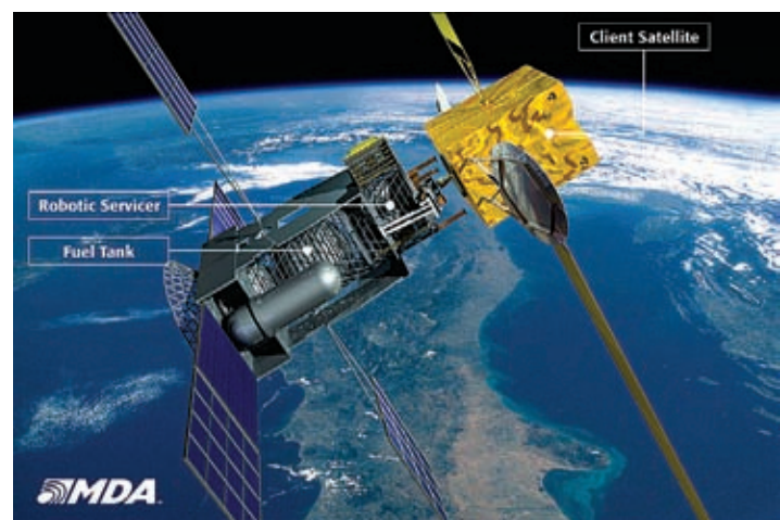
MDA's space infrastructure servicing concept involves a single satellite that would refuel, tow, inspect, and perform simple repairs. The spacecraft would service about a dozen satellites before being restocked in orbit with fuel and other supplies, allowing it to continue operations. Credit: MacDonald, Dettwiler and Associates
