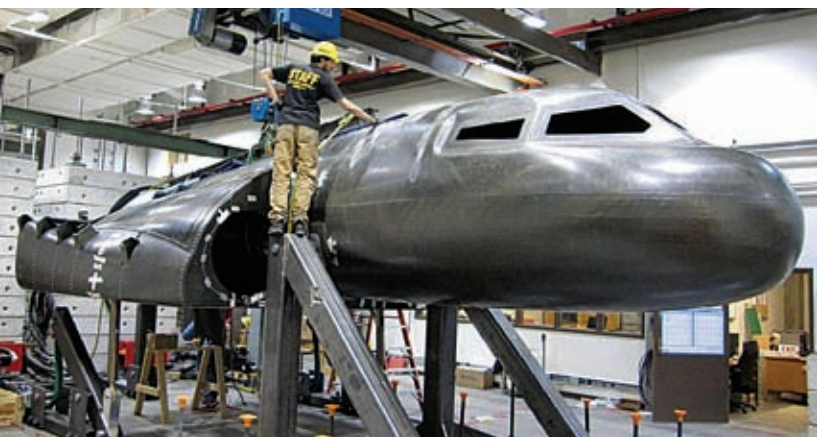
A technician works on the primary structure of Sierra Nevada Corporation's Dream Chaser spacecraft at the University of Colorado. As of February 2012, work was progressing according to the schedule in Sierra Nevada's CCDev agreement with NASA. Credit: Sierra Nevada Corporation
