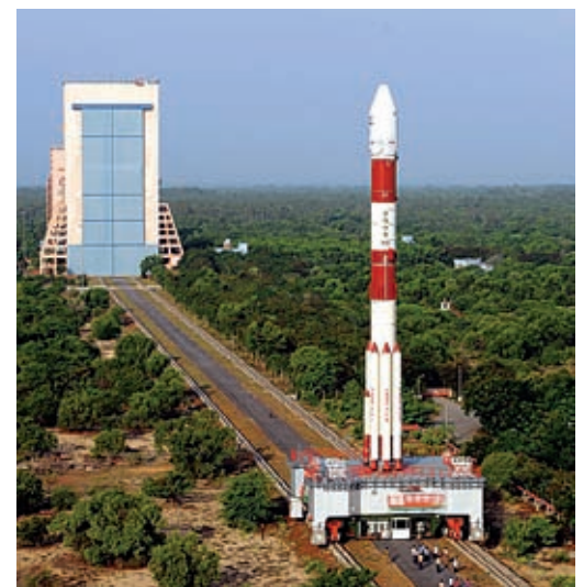
An Indian Polar Satellite Launch Vehicle is transported from the vertical integration building to the launch site. It successfully launched GSAT-12, an Indian communications satellite that will increase capacity for tele-education, telemedicine, and Village Resource Centres. Credit: ISRO
