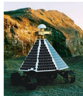
Astrobotic Technology is currently field testing lunar rover prototypes. The final rover will be remotely operated from Earth and will capture high-definition video and create a high-resolution terrain map as it explores. Credit: Astrobotic Technology
