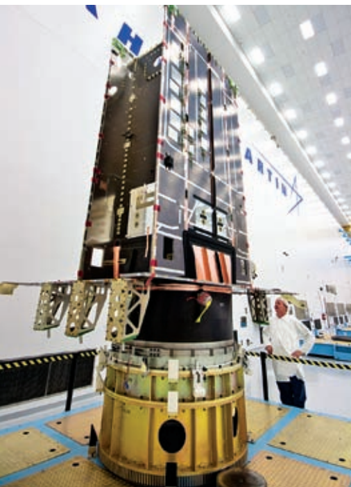
The core structure of the GPS III Non-Flight Satellite Testbed (GNST) stands in Lockheed Martin's GPS III Processing Facility. The GNST is a prototype that allows engineers to identify and solve issues prior to manufacturing the first space vehicle, reducing the overall cost of satellite production. Credit: Lockheed Martin
