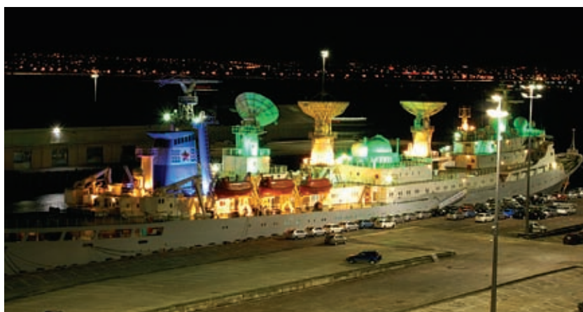
China's Yuanwang 2 tracking ship docks in New Zealand's Waitemata Harbor. Unlike nations that have access to a globe-spanning network of ground stations, China uses three Yuanwang-class tracking ships to monitor rocket launches and maintain contact with spacecraft. Credit: Abri le Roux
