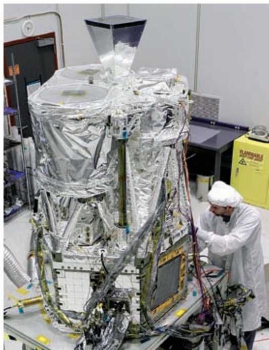
Workers at Orbital Sciences in Dulles, Virginia, prepare the integrated NuSTAR observatory, including the instrument and spacecraft, for environmental testing. This includes testing in a thermal vacuum chamber, ensuring the spacecraft can withstand the stresses of the space environment. Credit: NASA
