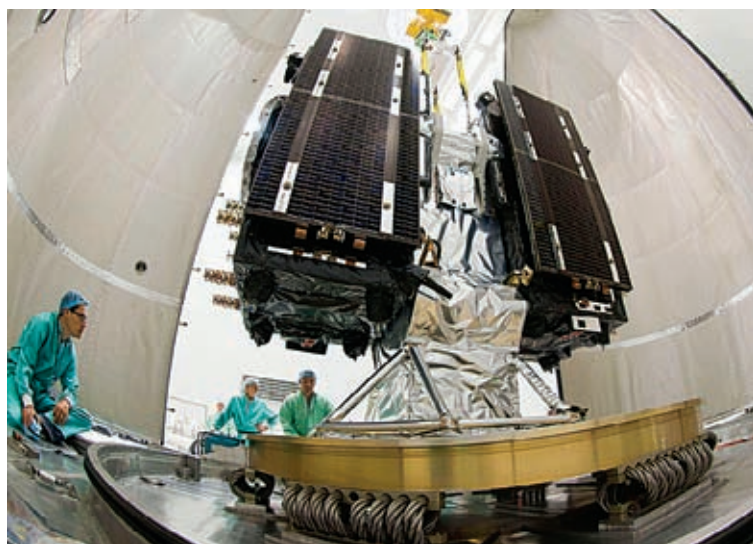
Twin Galileo satellites are attached to their support structure for launch atop the first Soyuz from French Guiana. The two satellites are part of the In-Orbit Validation phase that will test the Galileo system's space, ground, and user segments. Credit: ESA/S. Corvaja
