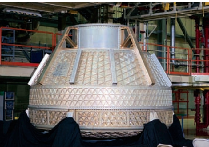
A pressure vessel for Boeing's Crew Space Transportation 100 (CST-100) spacecraft is displayed in Orbiter Processing Facility-3 at Kennedy Space Center, where manufacturing of the CST-100 will take place. Boeing chose to locate operations for the capsule here to benefit from close proximity to the launch site, pre-existing aerospace manufacturing facilities, and the experienced space workforce. Credit: NASA
