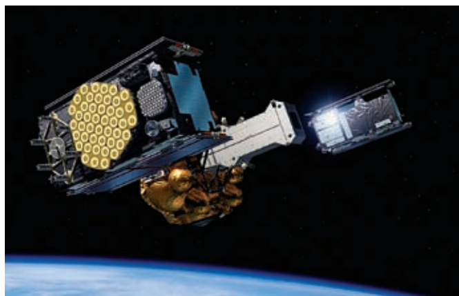
Launched in October 2011, two Galileo In-Orbit Validation satellites are simultaneously ejected from the upper stage of the Soyuz launcher. When complete, the global navigation system will consist of 30 satellites. The European Commission has worked to contain program costs by procuring satellites from two different providers. Credit: ESA/P. Carril
