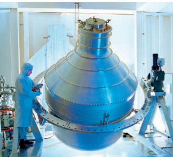
A 650-gallon Gravity Probe B thermal insulation vessel undergoes tests at Stanford University. It took Stanford, NASA, Lockheed Martin, and a host of physicists, engineers, and space scientists nearly 44 years to develop the ultra-precise gyroscopes and the other technology necessary to carry out this deceptively "simple" experiment. Credit: Lockheed Martin Corporation/R. Underwood
