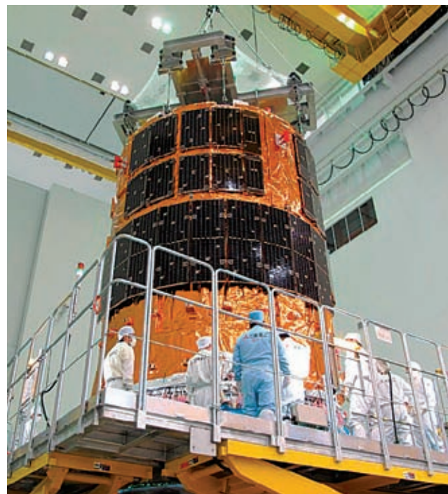
JAXA technicians prepare the H-II Transfer Vehicle "Kounotori." These transfer vehicles resupply the International Space Station, are loaded with waste material from ISS, then burn up upon re-entering the atmosphere. Credit: JAXA
