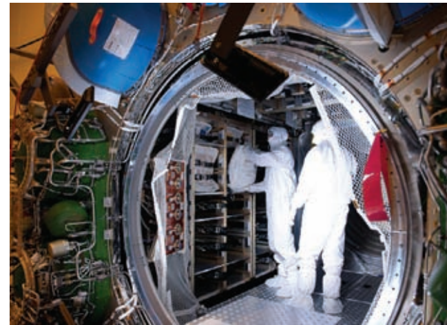
Technicians in Europe’s spacecraft in Kourou load cargo onto Automated Transfer Vehicle 3 for its journey to the International Space Station. The spacecraft carried 6,600 kilograms (14,540 pounds) of cargo, including propellant, oxygen, water, food, clothes, and equipment. Credit: ESA/CNES/Arianespace/Optique Vidéo du CSG/S. Martin
