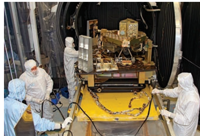
The Fine Guidance Sensor engineering test unit of the James Webb Space Telescope (JWST) is being prepared for cryogenic testing at a Canadian Space Agency Lab in Ottawa prior to delivery to NASA in mid-2012. The sensor enables precise pointing of JWST so that it can obtain high-quality images. Credit: CSA/COM DEV
