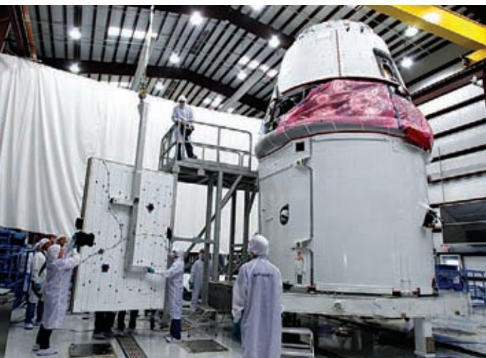
Technicians install Dragon's solar array panels at the SpaceX hangar in Cape Canaveral, Florida. The Dragon spacecraft will rely on solar arrays to provide power for running sensors, driving heating and cooling systems, and communicating with SpaceX's Mission Control Center and the International Space Station. Credit: SpaceX
