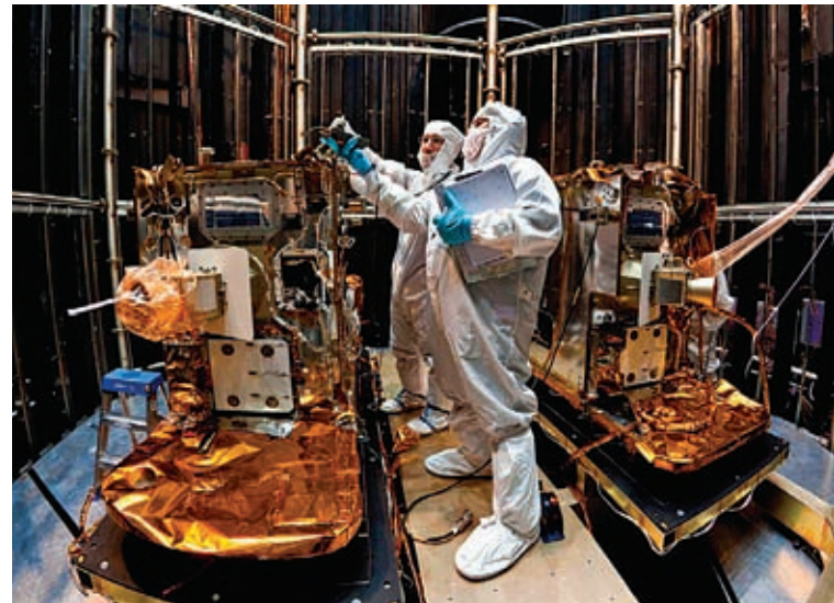
Technicians inspect GRAIL-A and GRAIL-B after testing in the vacuum chamber. The twin spacecraft underwent an 11-day-long test at Lockheed Martin Space Systems in Denver, Colorado, that simulated many of the flight activities they will perform during the mission, all while being exposed to extreme conditions that they will encounter in space. Credit: NASA/JPL-Caltech
