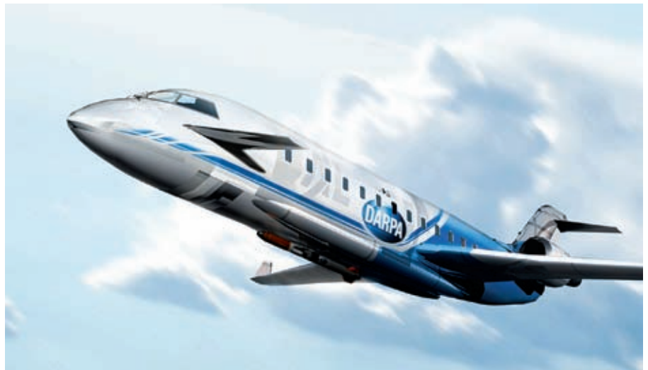
An artist's rendering of DARPA's Airborne Launch Assist Space Access concept. Similar to Orbital Sciences' Pegasus system, the rocket is attached to the belly of an airplane and released at a specified height. Credit: DARPA
