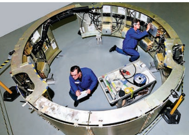
Technicians with ATK Aerospace Systems of Magna, Utah, make final preparations for testing inside an avionics mounting structure. The avionics system in a launch vehicle is responsible for controlling key guidance, launch, navigation, and recovery hardware. Credit: ATK
