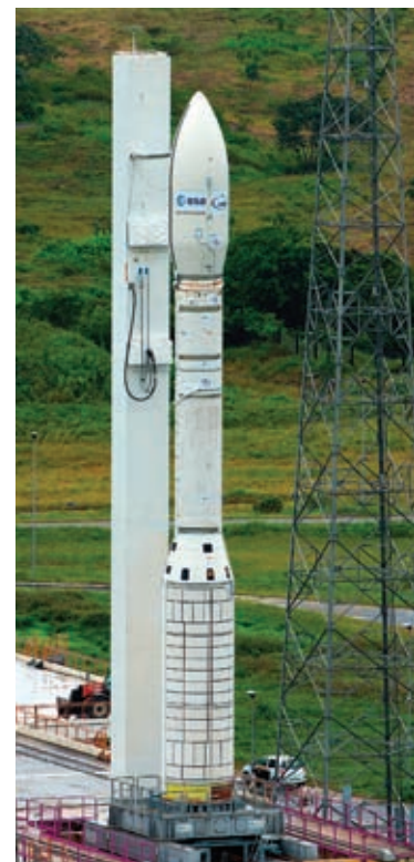
The first flight of the new Vega launch vehicle took place in February 2012 from French Guiana. Vega is designed to place satellites weighing 300–2,000 kilograms (660–4,400 pounds) into the polar and low Earth orbits used for many scientific and Earth observation missions. Vega can be configured to launch payloads ranging from a single satellite up to one main satellite plus six microsatsellites. Credit: ESA/S. Corvaja
