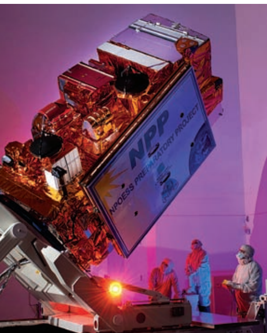
The Suomi National Polar-orbiting Partnership (NPP), a 2,100-kilogram (4,600-pound) spacecraft about the size of a small school bus, was launched in October 2011. The spacecraft carries five instruments that will contribute important information for weather forecasting. Credit: Ball Aerospace
