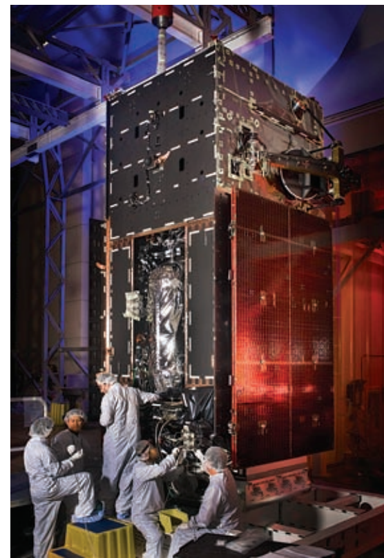
Lockheed Martin engineers complete work on the Space Based Infrared System (SBIRS) GEO-1 spacecraft. SBIRS provides infrared surveillance capabilities that aid in missile warning and defense and battlespace awareness. Credit: Lockheed Martin
