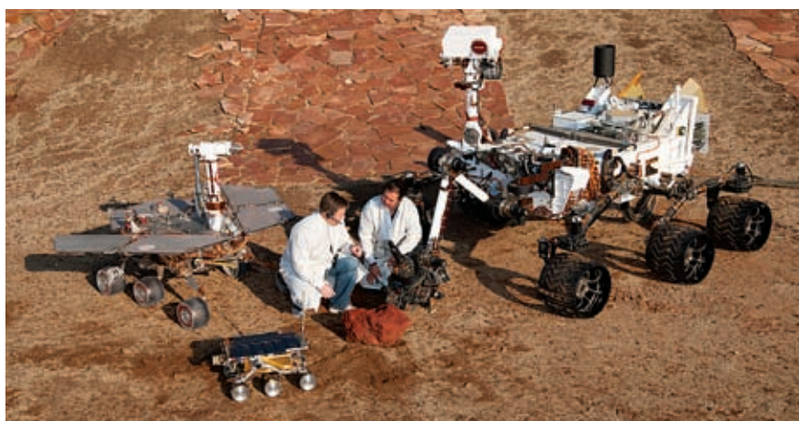
Mars rovers built by NASA’s Jet Propulsion Laboratory come together for a family portrait along with two spacecraft engineers. From left to right are the Surface System Test Bed rover, a working sibling of Spirit and Opportunity; Marie Curie, the flight spare for the Sojourner rover; and the Vehicle System Test Bed rover, which will be used to test commands before they are sent to Curiosity. Credit: NASA/JPL-Caltech
