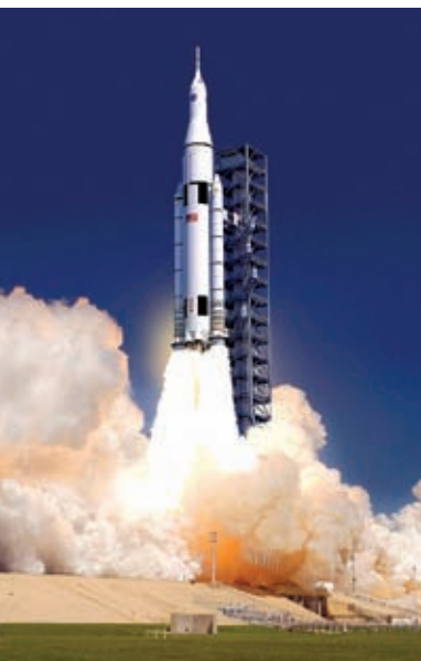
The SLS will use a liquid hydrogen and liquid oxygen propulsion system, with Space Shuttle Main Engines already in stock providing the core propulsion and the J-2X engine, now in testing, planned for use in the upper stage. This architecture enables NASA to leverage existing capabilities and keep development costs down. Credit: NASA
