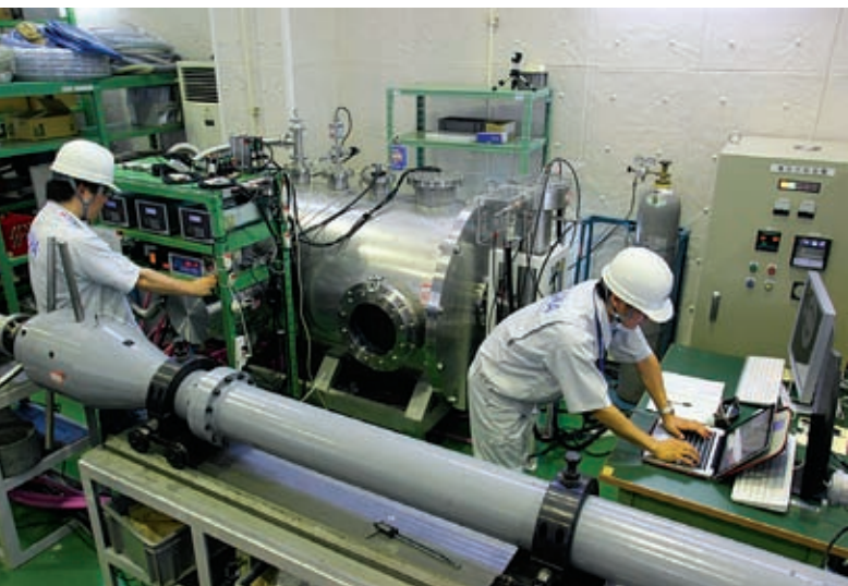
JAXA engineers examine the results of a test using the High Enthalpy Shock Tunnel, which simulates the environment experienced by spacecraft re-entering the atmosphere. During re-entry, vehicles can be exposed to temperatures higher than 10,000 degrees Celsius (180,000 degrees Fahrenheit). Credit: JAXA
