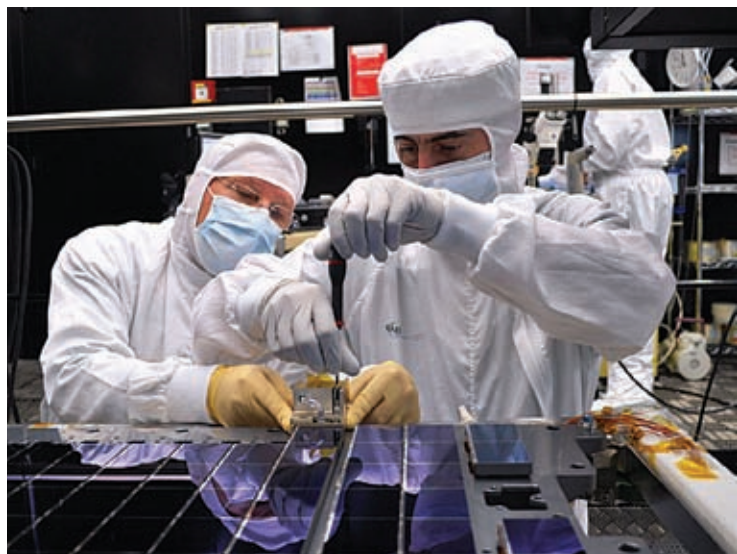
Technicians from Astrium, the Gaia mission's prime contractor, carefully construct one element of the spacecraft's imaging equipment at the company's facility in Toulouse, France. Each image captured by the camera will have around one billion pixels, the largest of any space mission to date. Credit: Astrium
