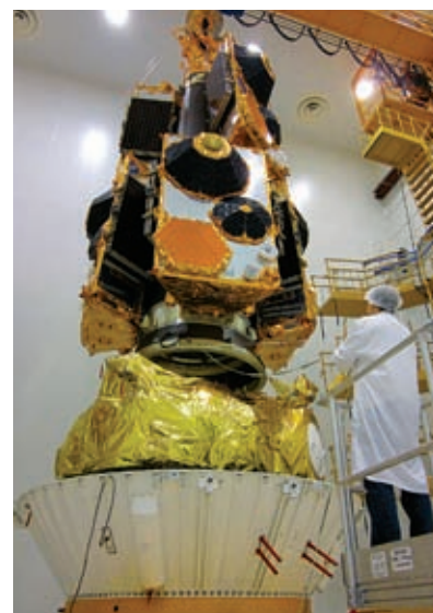
A dispenser with six Globalstar satellites is attached to the upper stage of a Soyuz launch vehicle inside the pre-launch facility at the Baikonur Cosmodrome in Kazakhstan. Credit: Arianespace
