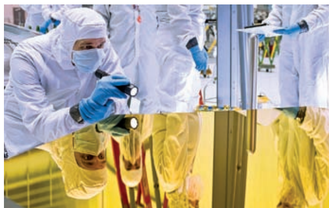
Technicians working on the James Webb Space Telescope inspect the prototype of a primary mirror segment. The telescope has a mirror more than twice the diameter of the one on the Hubble Space Telescope, allowing it to look further back in time to when galaxies were very young. Credit: NASA/Chris Gunn
