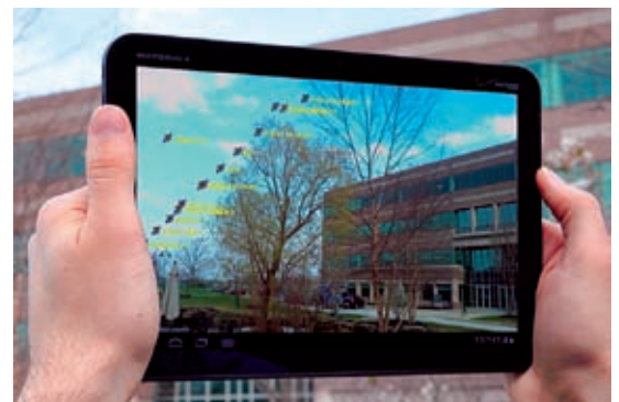
An application for phones and tablets running the Android operating system, Satellite AR offers an "augmented reality" experience that shows the user where spacecraft are in the sky. The user can zoom in for a closer view, touch a satellite icon on the screen for more detailed information, or plot an orbit as a ground track on Google Maps. Credit: AGI
