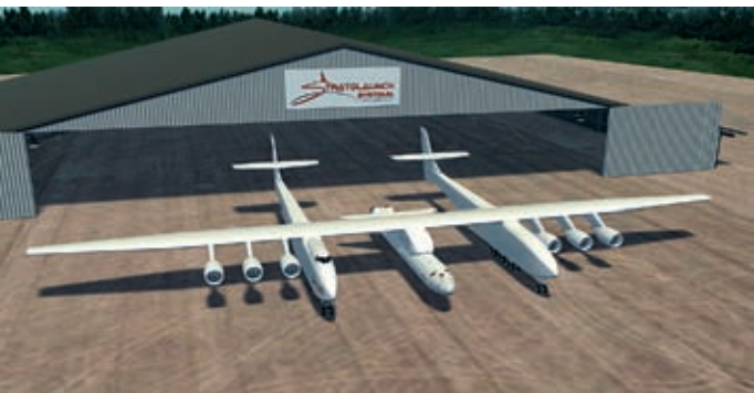
This rendering of the Stratolaunch Systems launch vehicle shows a multi-stage booster attached to the center of its carrier aircraft. The system is designed to deliver payloads of up to 4,500 kilograms (10,000 pounds) into low Earth orbit. Credit: Stratolaunch Systems
