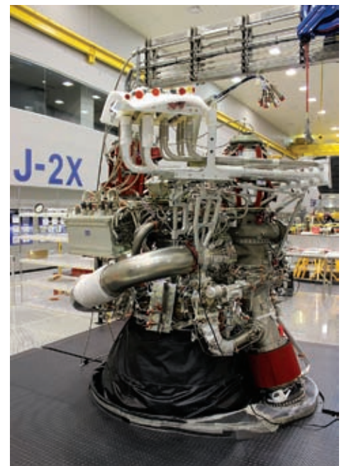
A J-2X rocket engine sits ready for testing in the assembly area at Marshall Space Flight Center. Designed to loft a launch vehicle's upper stage beyond low Earth orbit, the J-2X is built on decades of NASA spaceflight experience and technological advances. Credit: NASA
