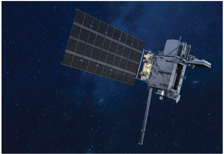
A rendering of the GOES-U satellite, launched in June 2024, which carries the Compact Coronagraph (CCOR) instrument to better monitor solar activity.
